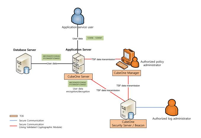
[Figure 2] API Operational environment of the TOE
